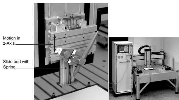
**Figure 1. Flatbed machine iselGFY44/48 with assembled pen carrier that is used in the synthesis of writing traces.**
