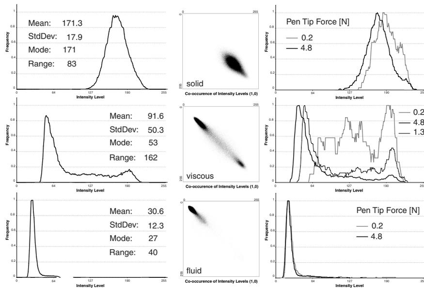
**Figure 3. Average intensity frequency plots and co-occurrence matrices (distance (1,0)) for solid, viscous and fluid ink types are given on the left and middle, respectively. On the right, frequency plots for single traces produced with varying maximal pen tip forces are shown.**
