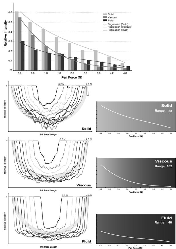
**Figure 4. Derivation of Ink-Deposition Models for solid, viscous and fluid ink type: Lower 10%-Quantil of intensity surface plots of ink traces written with variable pen tip forces were analyzed. Further on, the analytic regression results considering relative ink intensity as function of applied pen tip force (equation 10 - 12) and ink type specific distribution ranges.**
