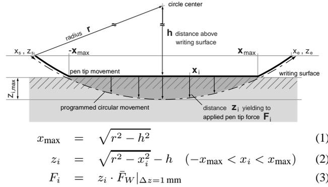
**Figure 2. Programmed circular movement for the analysis of ink deposit. Functional relations are given in equations 1-3.**
